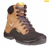
Ranger with reinforcement dedicated to the construction world Upper: Grain leather coated in PU - Bovine leather | Lining: Textile - Mesh - 3d - Breathable | Insole : EVA - Polyester | Outsole : Injected - PU - 2d | Reinforcements : Leather - PU | Anti-perforation insert : Stainless steel | Security toe-cap : Composite | Lacing system : Laces | Weight : 740 g per shoes
