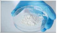
D Optional test of EN149: 2001 standard for clogging of dolomite dust.
